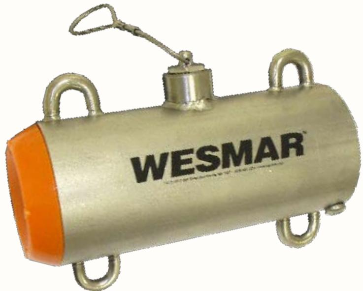
The reliable and sturdy WESMAR CS20 Catch Sensors measure the fill rate of the trawl, alerting you when the codend is full. These lightweight, high-frequency sensors are factory programmed to operate with any WESMAR trawl sonar or with other trawl sonar.
