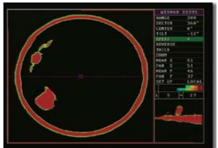
The SS395 in 360 degree view of bottom with fish to port. Thickness mode isolates the fish in lower right-hand screen.
