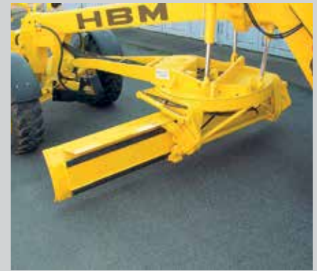
Sophisticated kinematics for rapid adjustment of the desired blade position.
