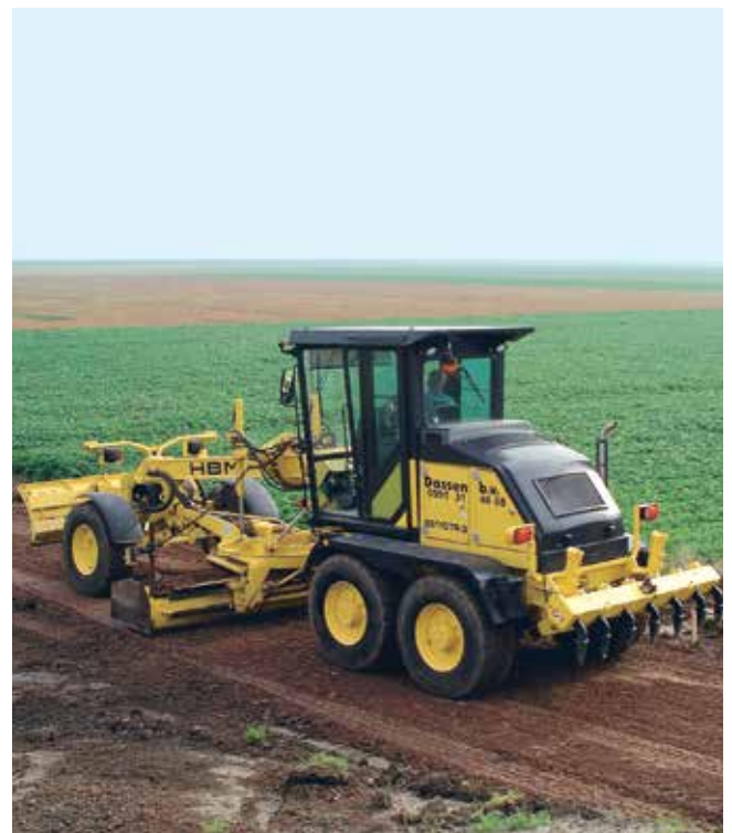
BG 110 TA-4, the compact tandem grader, ideal for small and medium building sites
