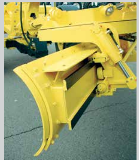
Infinitely adjustable hydraulic cutting angle adjustment.
