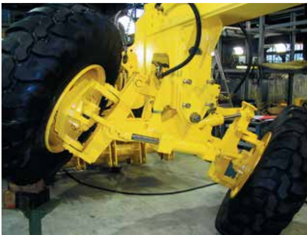
Driven front axle with wheel lean.
