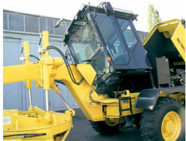
Good maintenance accessibility: Cab and engine cover tiltable.
