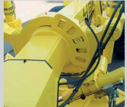
Adjustable turning bridge for embankment and trench work.
