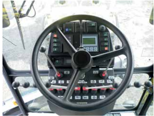
Good view to all sides with adjustable Euro, NAIS (rods) or joystick controls available.
