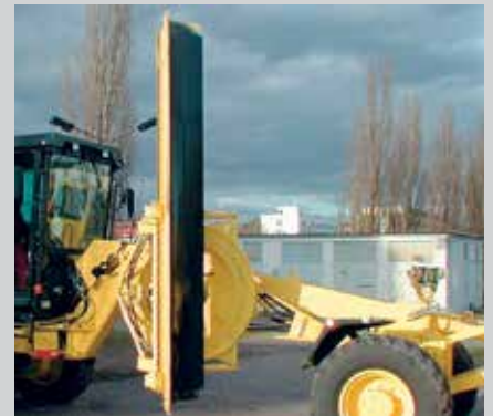
Closed turning circle available with roller bearings. Ground clearing angle 90° to the right and left.
